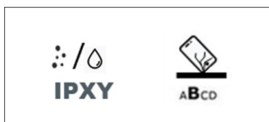
Figure 2: Currently planned pictogram for dust / water protection (left) and pictogram for free fall reliability (right)
